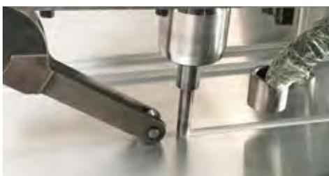
Joining the metal using the FSW technology
