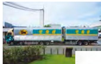
A full view of a new standard dry van type full trailer truck
